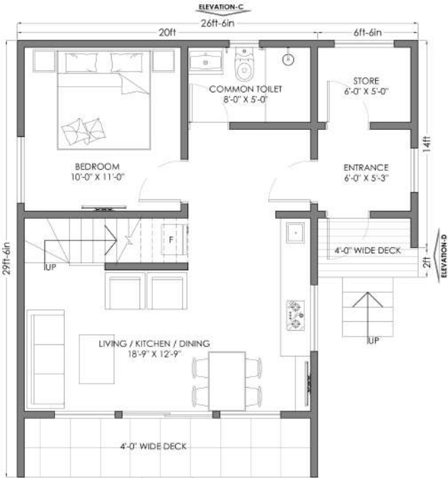
BARN HOUSE - 2A GROUND FLOOR PLAN COVERED AREA = 681 Sq.Ft DECK AREA = 13 Sq.Ft TOTAL BUILT UP AREA = 1284 Sq.Ft
