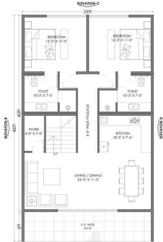
CABANA 'A' - 3BHK GROUND FLOOR PLAN COVERED AREA = 1196 Sq.Ft BUILT UP AREA = 1664 Sq.Ft
