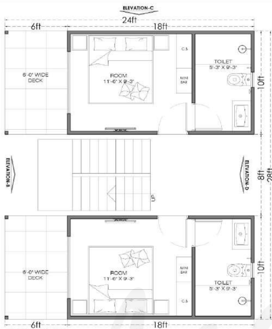
4ROOMS COTTAGE GROUND FLOOR PLAN COVERED AREA = 480 Sq.Ft STAIR AREA = 120 Sq.Ft TOTAL BUILT UP AREA = 1080 Sq.Ft
