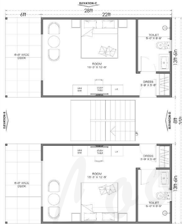
4ROOMS COTTAGE GROUND FLOOR PLAN COVERED AREA = 756 Sq.Ft STAIR AREA = 120 Sq.Ft TOTAL BUILT UP AREA = 1632 Sq.Ft
