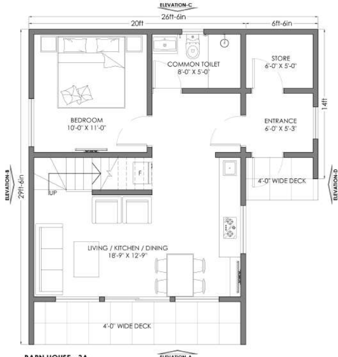
BARN HOUSE - 3A GROUND FLOOR PLAN COVERED AREA = 681 Sq.Ft TOTAL BUILT UP AREA = 1271 Sq.Ft
