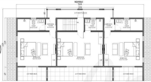
FIRST FLOOR PLAN COVERED AREA = 1348 Sq.Ft COVERED DECK AREA = 336 Sq.Ft
