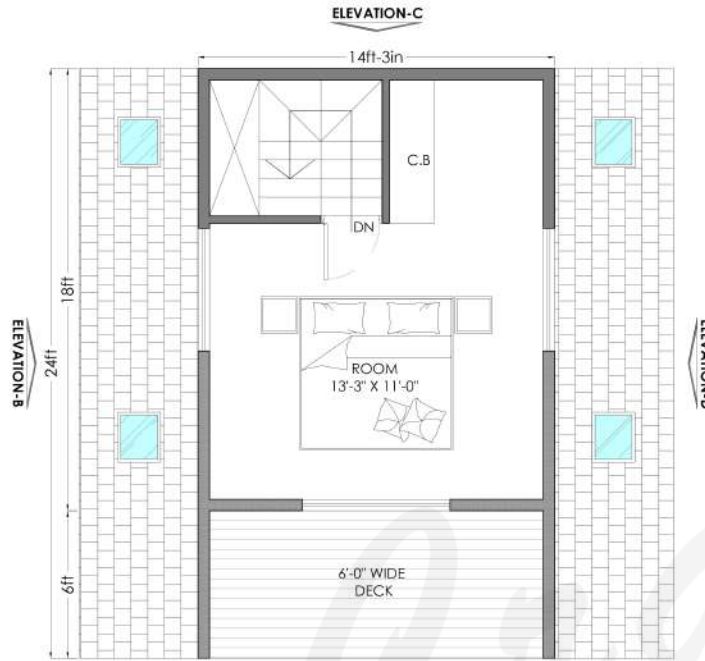
FIRST FLOOR PLAN COVERED AREA = 342 Sq.Ft
