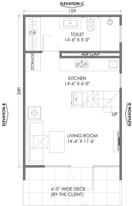
MODROOM-XL LOFT ELEVATION-A GROUND FLOOR PLAN COVERED AREA = 360 Sq.Ft TOTAL AREA = 620 Sq.Ft
