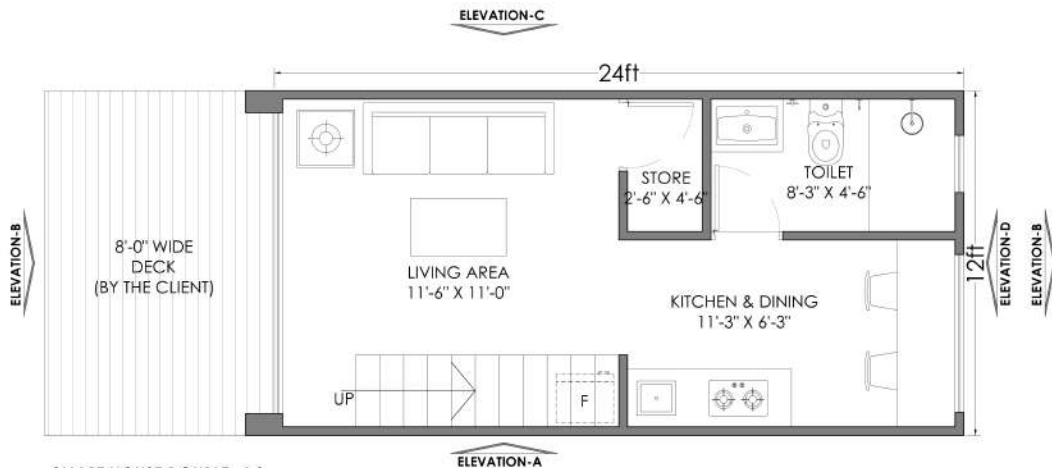
SMART HOUSE DOUBLE -A4 GROUND FLOOR PLAN COVERED AREA = 288 Sq. Ft TOTAL BUILT AREA = 432 Sq. Ft
